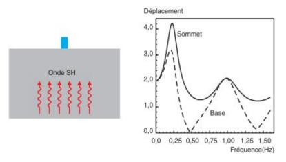
**Figure 4.-** Soil-structure interaction model considered (left); dimensionless displacements at the base and at the top of the structure as a function of frequency (right) (Semblat et al, 2005) [10].
