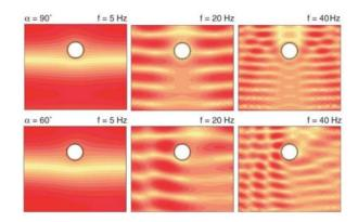
Figure 8.- Iso-displacements areas for vertical incidence and incidence of 60 degrees to the horizontal and for three different frequencies. (Semblat et al, 2005) [10].
