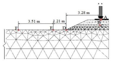
Figure 12.- Finite element mesh and points considered for the 2D PLAXIS model (Shahraki et al, 2014) [3]
