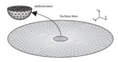
Figure 2.- Border Element Modeling of 3D Seismic Wave Propagation: Hemispheric Sedimentary Basin Model (Dangla et al., 2005) [9].
