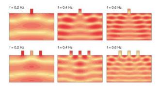
Figure 5.- Movement of soil and structures at different frequencies (Semblat et al, 2005) [10].
