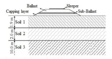
Figure 11.- Model geometry in 2D modeling (Shahraki et al, 2014) [3].
