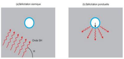
Figure 7.- Tunnel subjected to an SH (a) seismic wave or to a point excitation (b) (Semblat et al, 2005) [10].
