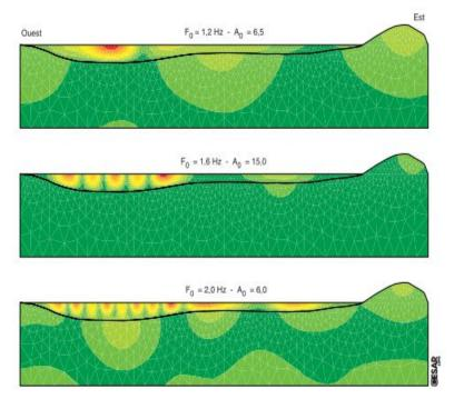
**Figure 1-** Border element modeling of the amplification of seismic waves in the center of Nice: amplification factor  $A_0$  at different frequencies  $F_0$  (Semblat et al, 2000) [8].
