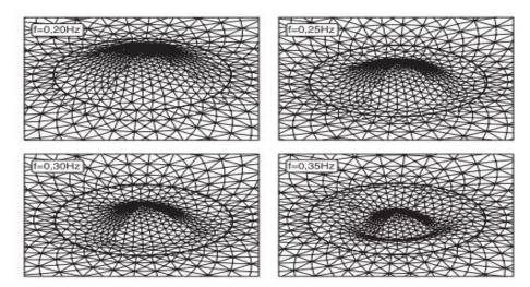
**Figure 3.-** Border element modeling of three-dimensional seismic wave propagation: deformation of the sedimentary basin at different frequencies (Dangla et al., 2005) [9].
